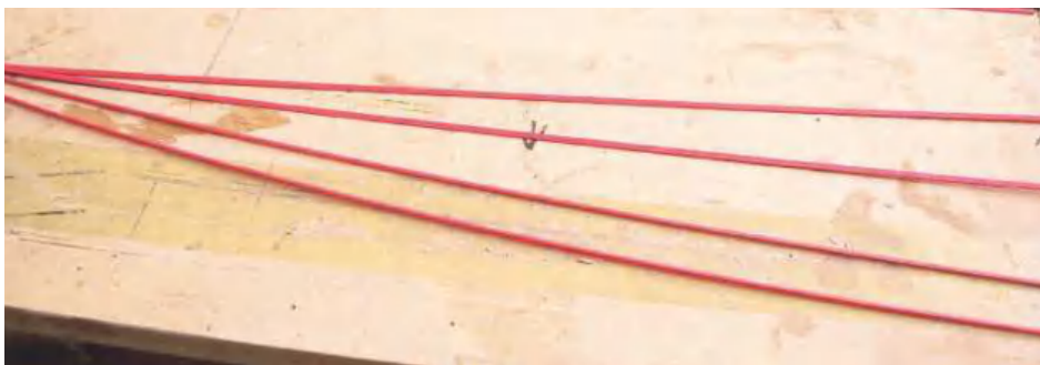
STEP 3. Veneer strips are prepared for the rosette
